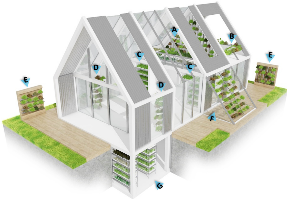
Figure 2. Examples of locations for integrating home hydroponics into buildings. A, attic; B, terrace; C, inserted into a wall; D, mobile appliances; E, outdoor wall; F, greenhouse; and G, basement.
